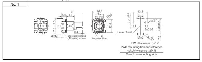
Standard rotation-torque / Bushing Type with Sleeve / with Switches ......With detents : EVEJBE
