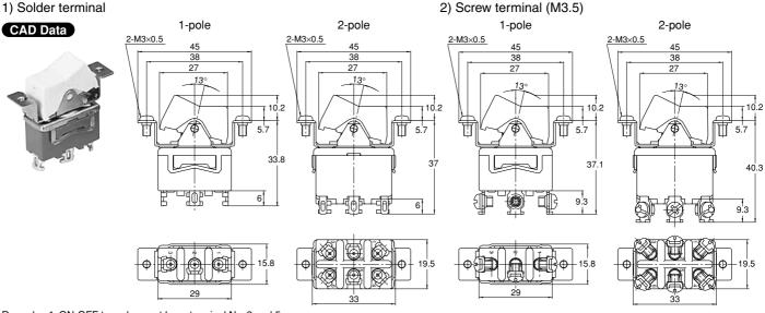
Remarks: 1. ON-OFF type does not have terminal No. 2 and 5. 2. Dimensions of actuator:  $13.4 \times 27$
