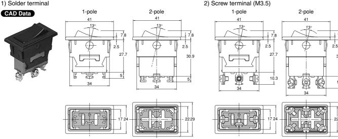
Remarks: 1. ON-OFF type does not have terminal No. 2 and 5  $\,$ 2. Dimensions of actuator: 1-pole: 12.6  $\times$  29, 2-pole: 17.4  $\times$  29
