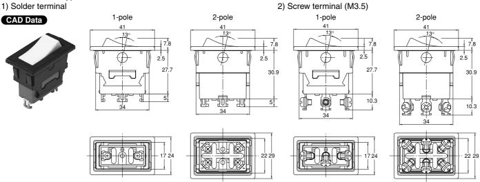
Remarks: 1. ON-OFF type does not have terminal No. 2 and 5. 2. Dimensions of actuator: 1-pole: 12.6  $\times$  29, 2-pole: 17.4  $\times$  29
