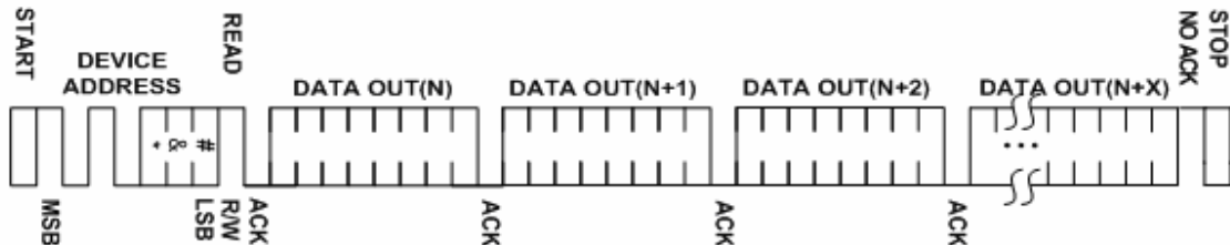
Figure 7: SEQUENTIAL READ (SDA INPUT/OUTPUT)
