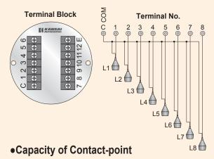
The capacity at the contact, described in the standard specification, shows that of Kari Mini Float Switch alone. As for the common specification(Standard), make sure that the total current capacity is less than 3A before your use. When it exceeds 3A, you should use either a supplemental elay or select an independent-contact type.
